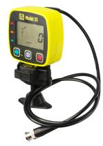
An internal switch is used to enable or disable the front-panel setup feature to protect desired settings from inadvertent modification. Setup is also available via software available from Ludlum Measurements.
